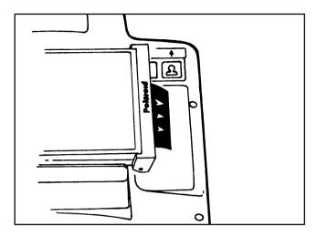
4 Pull the black paper tab out of the camera back, keeping the tab perpendicular to the camera at all times. The best method is to place the camera on a flat surface, grip the camera with your left hand and pull the tab with your right hand. This ensures that the film in the camera remains aligned.
